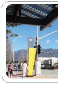
In addition to providing shade and shelter to pedestrians, the system is expected to generate 30,000 kilowatt-hours of clean energy annually, Mejia said, which is the equivalent power use of six typical Pasadena homes. All energy from the BIPV is fed to PWP's citywide power grid, but counts as a 25 percent offset of the station's power use.
