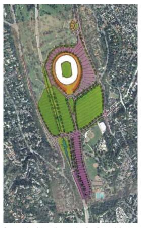
Reorganization of the parking around the Rose Bowl could include a realignment of the stadium entry road to allow more efficient use of adjoining spaces; impervious parking surfaces with reinforced turf to support parking, recreation, and stormwater harvesting; and improved parking flow and striping layouts to maximize use on large event days.
