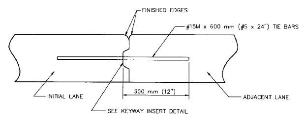
CONTACT JOINT WITH KEYWAY AND TIE BAR
